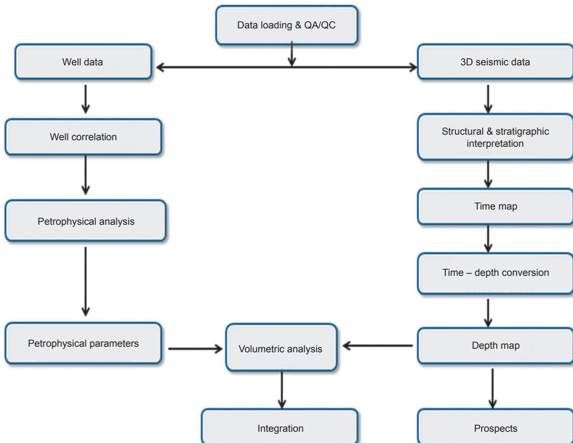
**Fig. 7. Workflow for evaluation phase**
