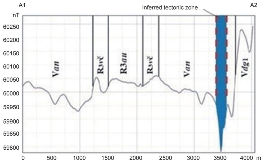
**Fig. 3. Graph of the magnetic total field modulus along the profile A1–A2 with preselected value ranges**
