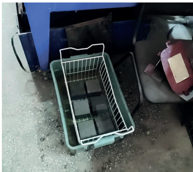
Fig. 1. Freeze-thaw cycle with concrete samples:
