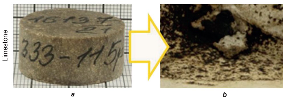
Fig. 5. Changes in the structure of the carbonate core before (a) and after (b) acidizing
