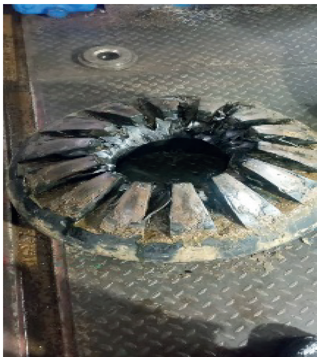
Fig. 3. Damaged sealing element (photo made by the authors of the article):
